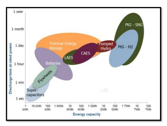
**Storage Capacity and Discharge times of different storage technologies** From: (Electrification Strategy EU, 2022)
